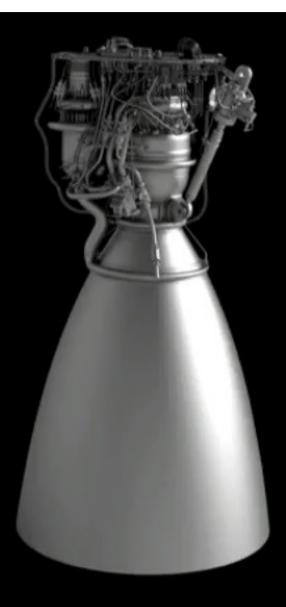
Cycle Full-flow staged combustion
