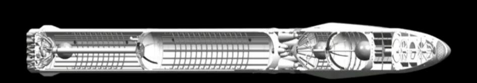
Carbon-fiber primary structure Densified CH<sub>4</sub>/02 propellant Autogenous pressurization
